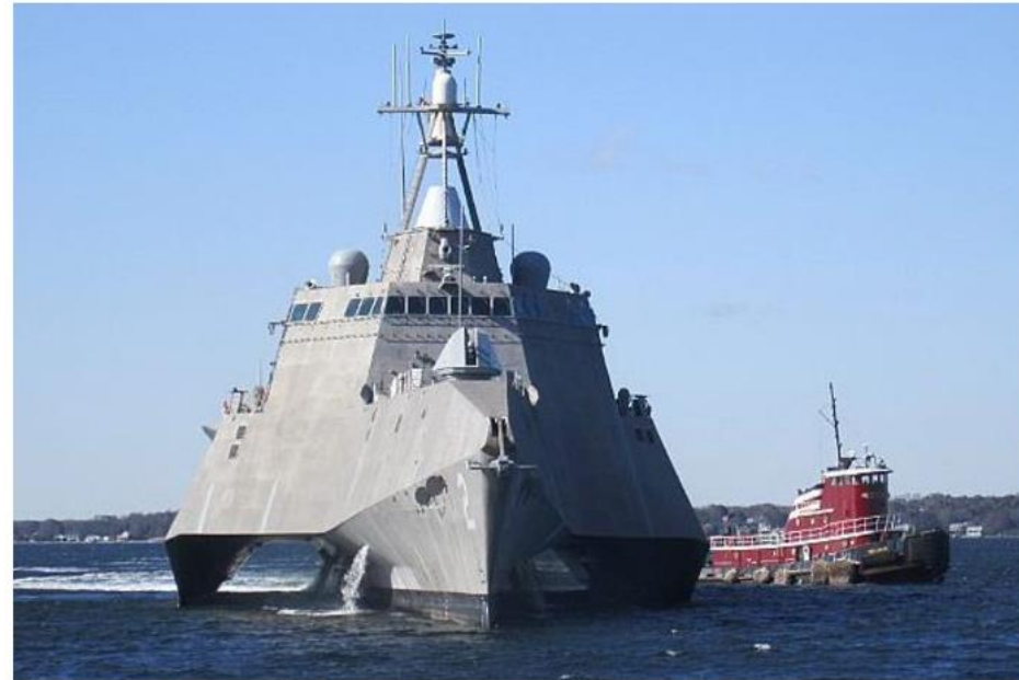
LCS-2, USS Independence, shows off its unique "trimaran" design.
